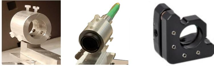
**Figure 5.21:** Actual collimator holder (left), when holding the collimator (center) and commercial kinematic mount that can be more suited to hold and adjust the inclination of the collimator (right)<sup>1</sup>.
