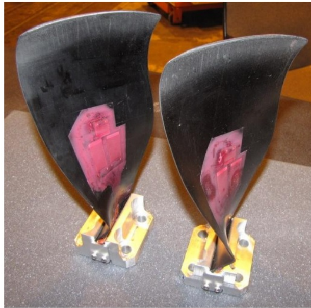
Figure 1.15: General Electric Aviation (GE) subscale composite fan blades with piezoelectric patches for the implementation of active control system [8].
