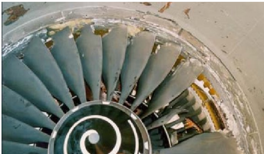
Figure 1.4: Fan blade failure due to a high cycle fatigue of the blades [3].
