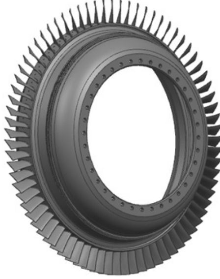
Figure 1.3: A CAD view of the monobloc bladed drum (i.e. BluM).
