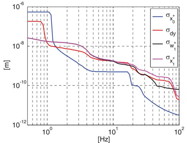
Figure 4: Integrated RMS for  $k_g = 3e8N/m$ .
