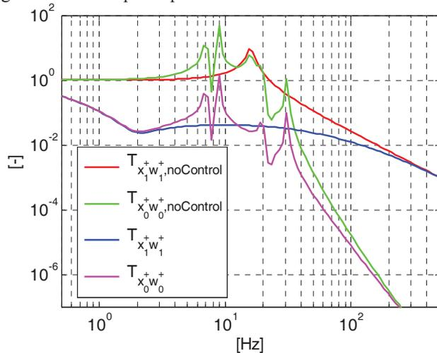
Figure 10: Transfer functions between the ground and the quadrupoles, with and without control.
