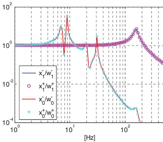
Figure 3: Transfer functions between the ground and the quadrupoles.
