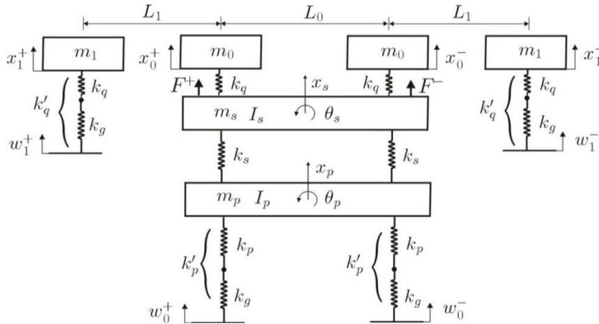
Figure 2: Lumped mass model of the ILC final focus with the SID configuration.
