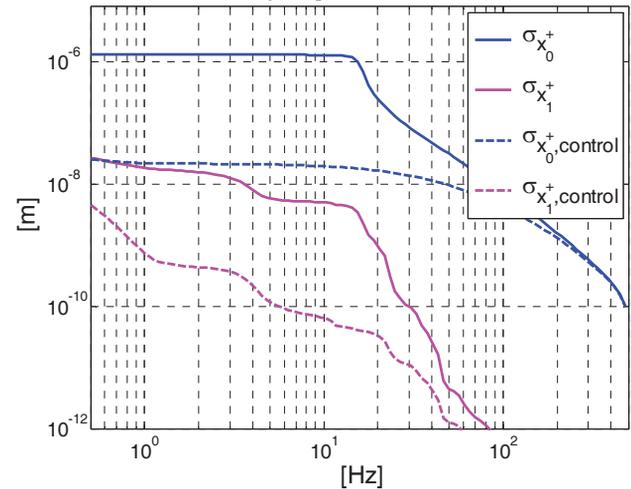
Figure 11: Integrated RMS when the control is turned on and off.
