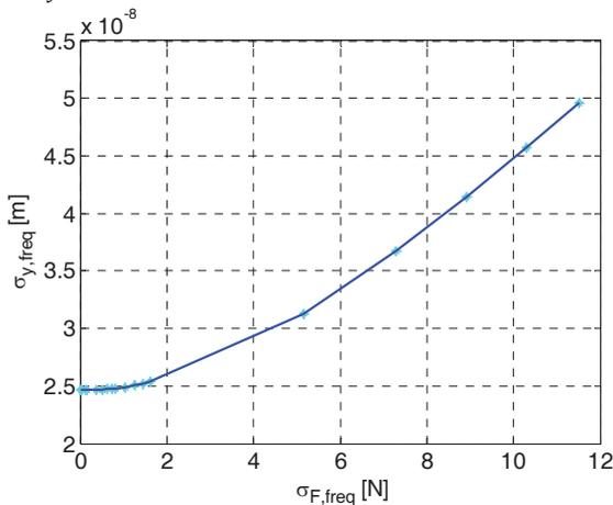
Figure 6: Evolution of the beam-beam offset at the interaction point  $\sigma_y$  at 5 Hz as a function of the amplitude of the technical noise on QD0
