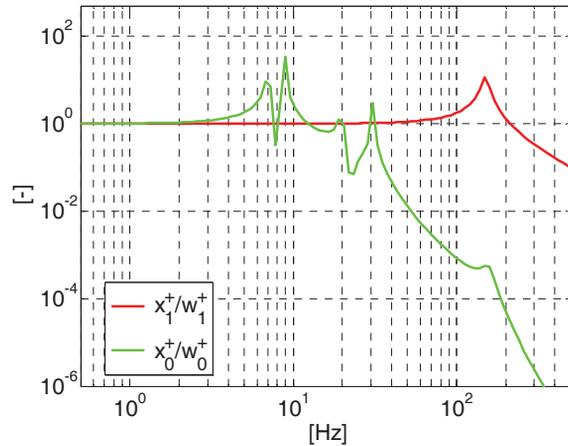
Figure 8: Transfer functions of the quadrupoles for  $f_{QF1} \approx 150Hz$  with  $\sigma_{F_2} \approx 0.02N$ .
