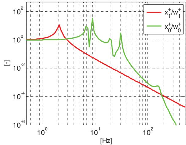
Figure 7: Transfer functions of the quadrupoles for  $f_{QF1} \approx 2Hz$  with  $\sigma_{F_2} \approx 0.02N$ .
