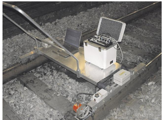
Fig. 4. Trolley for the measurement of rail corrugation [1].
