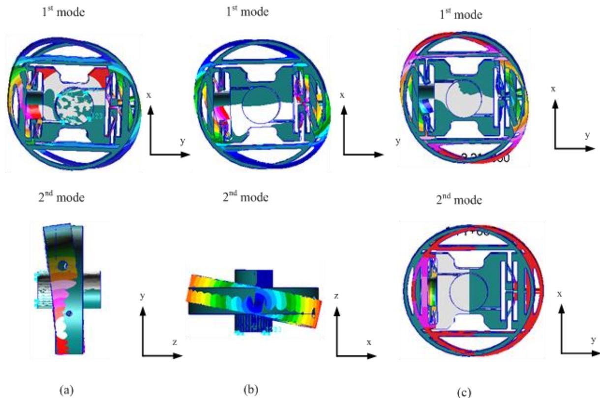
**Figure 3** The first two mode shapes of the inertia shaker for a piezo element with Young's modulus of 76.5 GPa (left), 5 GPa (middle) and 0.3 GPa (right).
