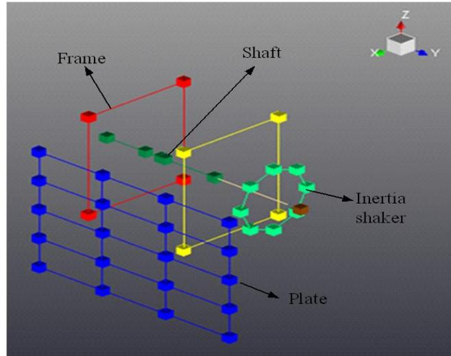
**Figure 4** Schematic representation of the measurement setup, with indications of the accelerometers attached to the structure at various components.
