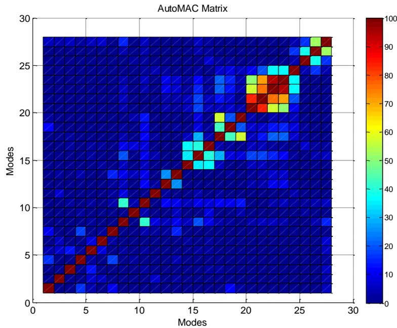
Figure 7 AutoMAC matrix between experimentally estimated modes
