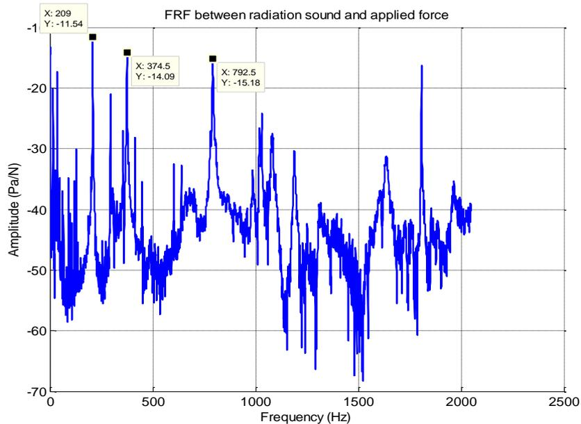
**Figure 6** FRF between the input force and the acoustic pressure measured close to the plate
