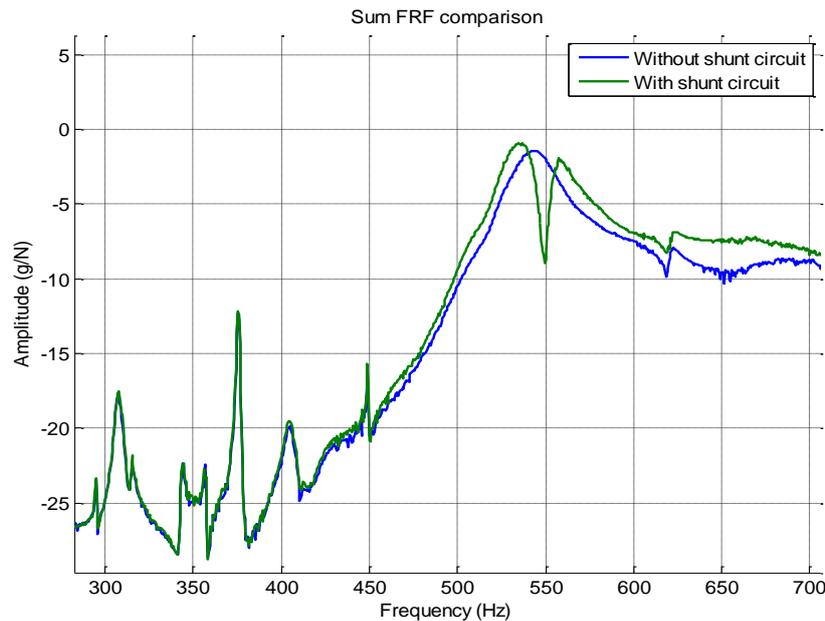
**Figure 9** A Comparison of Sum- FRFs with and without shunt circuit
