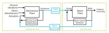
Figure 3: Block diagram of the final focus of a linear particle collider.
