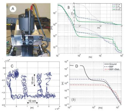
Figure 4: (a) Test bench; (b) Transmissibility between the motion of the ground and the quadrupole; (c) Illustration of the nano-positioning capability; Integrated RMS of the ground, the beam jitter with B(s), the beam jitter B(s) and Q(s).
