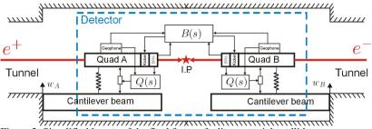
Figure 2: Simplified layout of the final focus of a linear particle collider.
