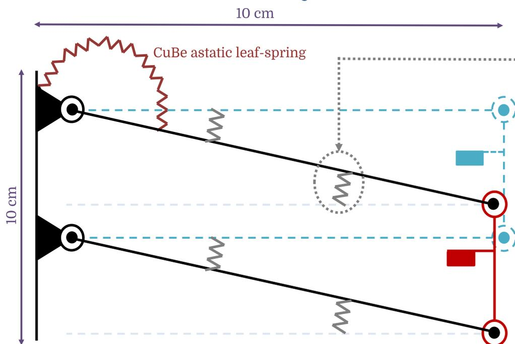
Fig. 2: Schematics of the mechanics of the sensor. The “four-bars” mechanism guarantee the translation motion of the mirror.
