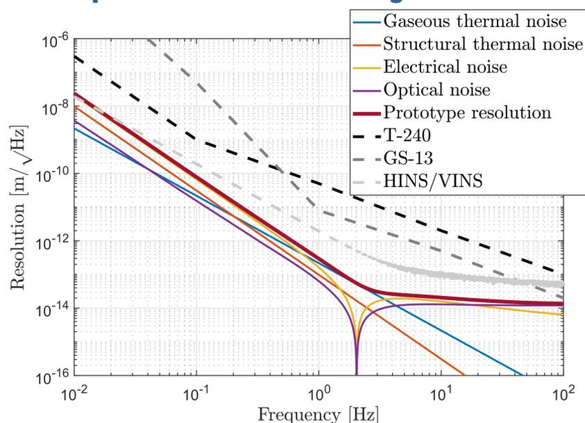
Fig. 5: Estimated noise budget of the prototype & comparison with previous sensors.
