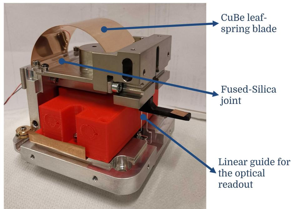
Fig. 1: Mechanics of the vertical inertial sensors with fused-silica joints.
