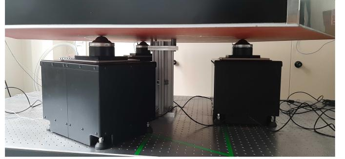
Fig. 7. Picture of the three isolators. A sphere is used to have the smallest contact point between the isolators and the hexagonal table. A guide is put at the centre of mass for safety reasons; there is no contact between the part connected to the hexagonal table and the part fixed to the bottom table except in case of accident.
