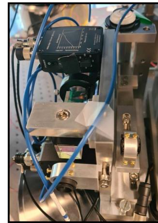
Horizontal Inertial sensor [4]
