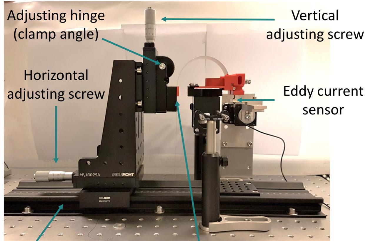
Adjusting hinge (clamp angle)
