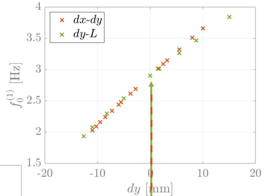
Curves very close: the effects of  $dx$  &  $L$  are lower than the one of  $dy$
